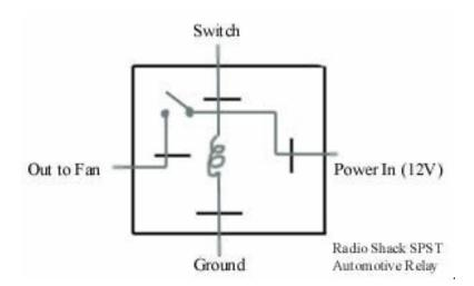
This is my wiring layout. The Radio Shack relay comes with a nice diagram, I just felt like making a little picture. When I flip the switch, power will go through the relay and to the cooling fan and output in the fuse box relay. This is ok, as I don't plan on turning on the switch if the cooling fan is already on. Since it's off, power isn't getting through the factory relay to blow any fuses. This is a little hard to explain, please read on.
